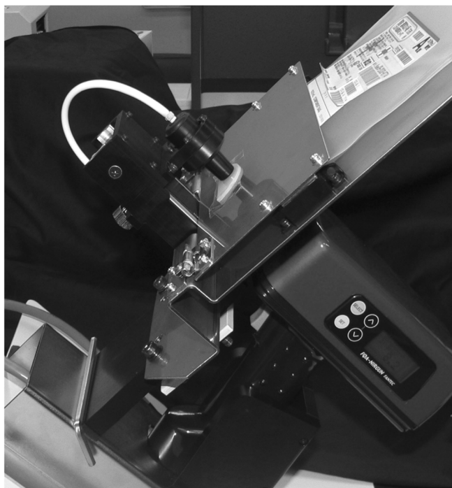
Figure 1. NIR measurement of platelet component using a portable NIR instrument.
