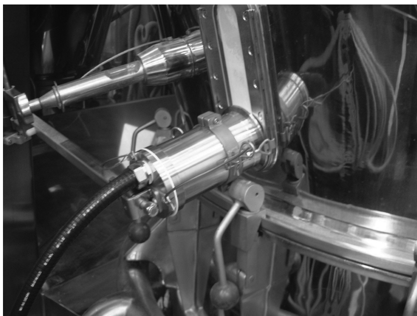
Figure 1. NIR Probe attached to fluid bed dryer.
