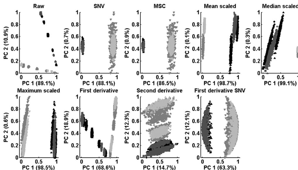
**Figure 3.** Score plots (PC1 vs PC2) of raw and pre-treated spectra. Colour code: samples in increasing order of brightness: blue cardboard cylinder, blue cardboard flat, pink paper cylinder and pink paper flat. Scores were scaled between 0 and 1.
