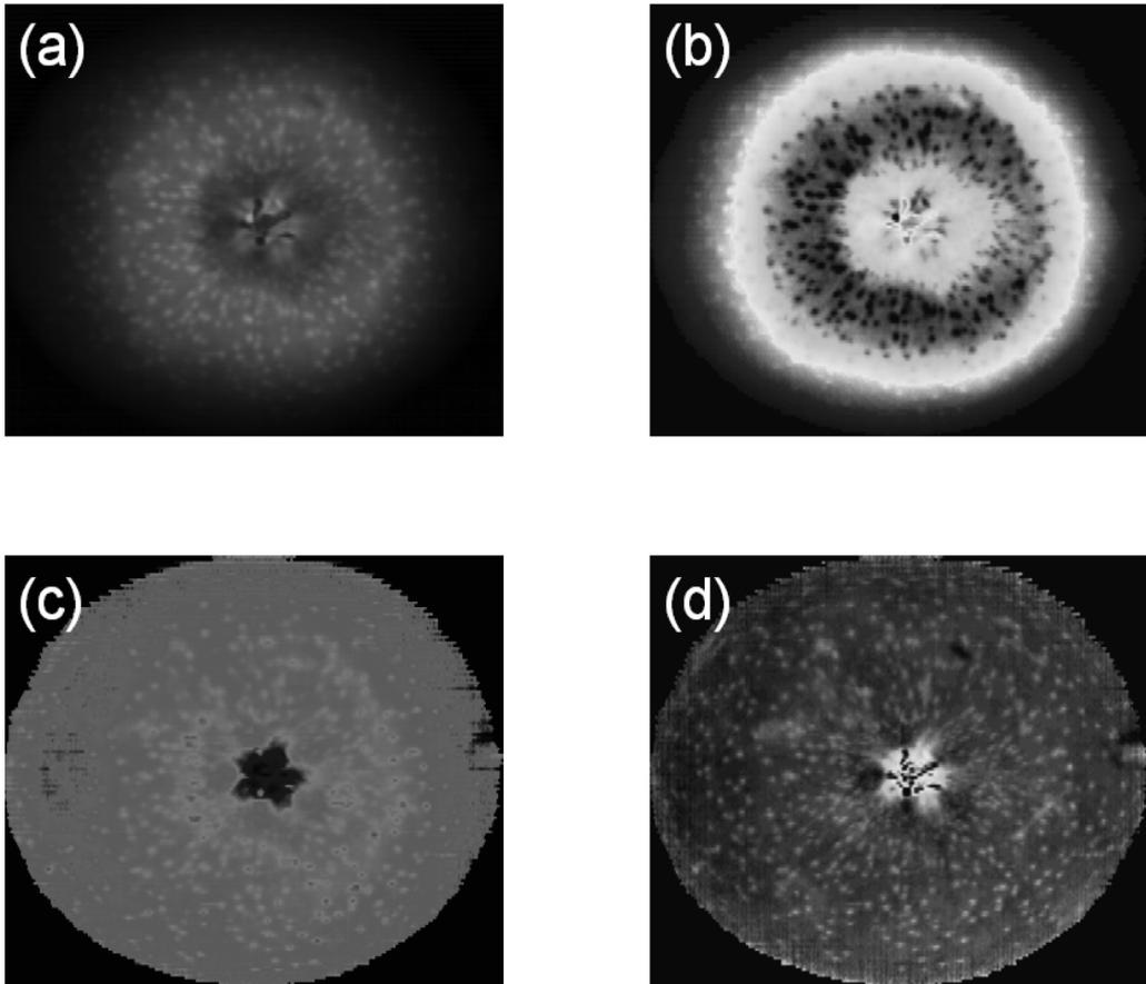
**Figure 1.** Apple hyperspectral image scanned 950–1650 nm. (a) grey scale image, in which it is possible to observe a shiny central ring and dark edge. (b) PC 1 score image of raw spectra. (c) PC 1 image of median normalised spectra. (d) PC 1 score image of SNV pre-treated spectra.
