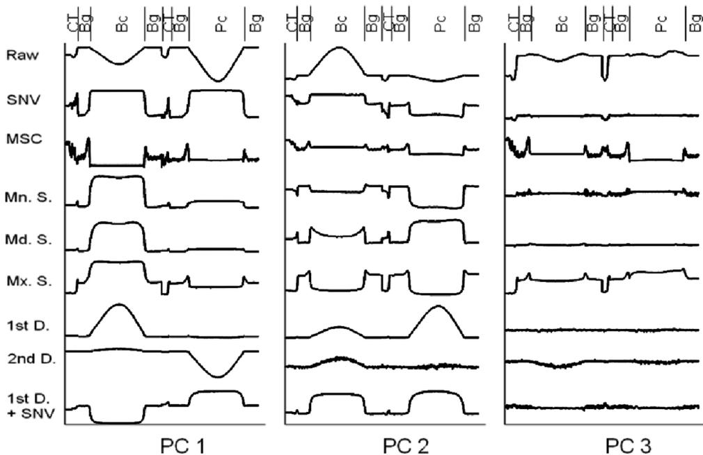
Figure 4. Score profiles of average raw and pre-treated spectra. CT = calibration tile; Bg = background; Bc = blue cylinder; Pc = pink cylinder. Scores were scaled between 0 and 1.
