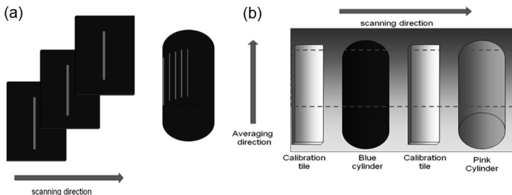
**Figure 2.** Principal component samples (a) sub-sampling areas from the three flat images and cylinders (b) region where the principal component analysis was performed and averaging direction to obtain the score profile.
