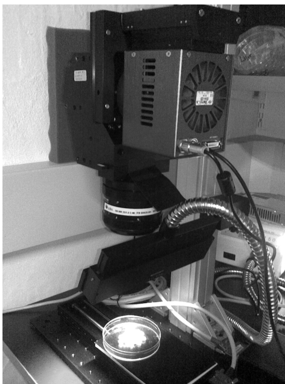
Figure 1. Acquisition of wheat kernels using the hyperspectral camera.
