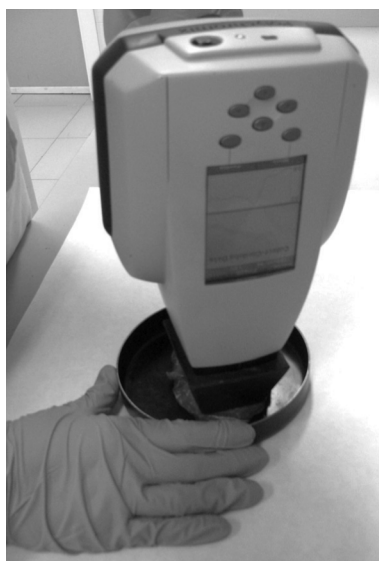
Figure 1. Measurement of NIR spectra on intact pork muscles.
