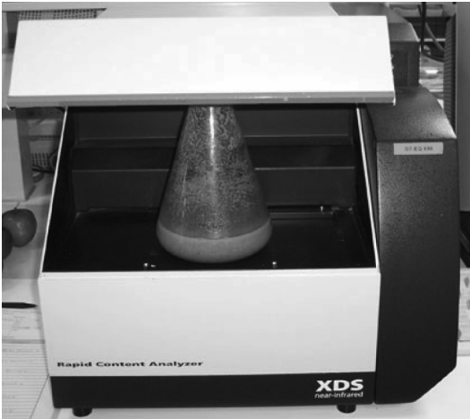
Figure 2. Erlenmeyer flask spectral acquisition directly on the sample window.
