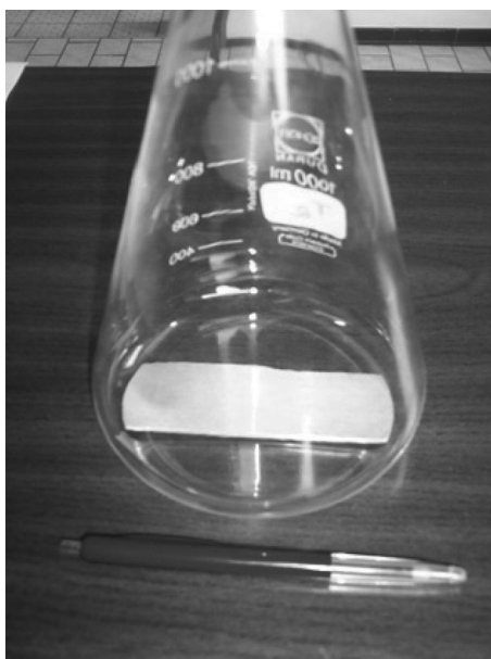
Figure 1. Erlenmeyer flask equipped with an aluminium plate used as reflector.
