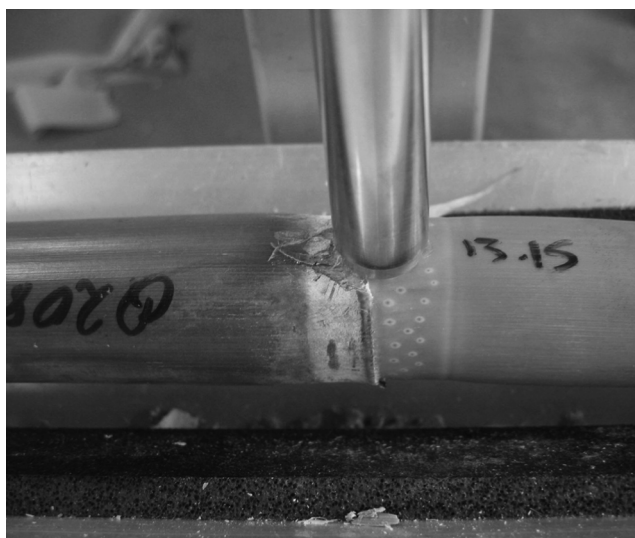
Figure 1. Obtaining an NIR spectrum of a sugarcane bud using a fibre optic probe assembly.
