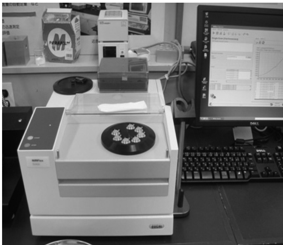
Figure 1. NIR spectrophotometer Model NIRFlex N500 (Buchi Labortechnik AG, Flawil, Switzerland) equipped with a six channel single kernel sample cells.
