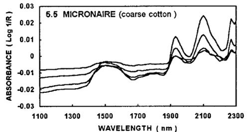
Figure 14. Transreflectance spectra for different bundle thicknesses using a coarse cotton.
