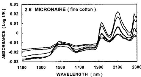
Figure 13. Transreflectance spectra for different bundle thicknesses using a fine cotton.
