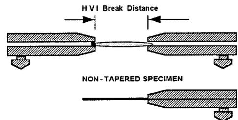
Figure 6. Sketch of non-tapered cotton fibre specimen preparation procedure.
