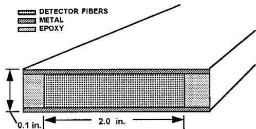
Figure 4. Sketch of optic fiber transmission detector probe.
