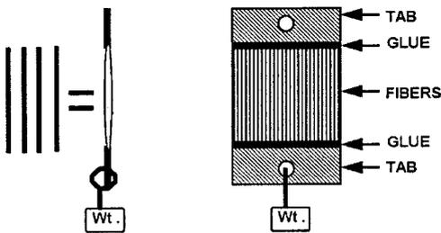
Figure 7. Sketch of cotton fiber tension experiment.
