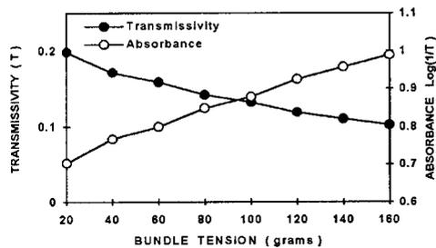
Figure 10. Light transmission data at 1550 nm.
