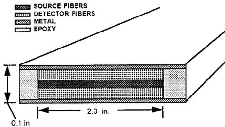
Figure 3. Sketch of optic fiber probe source.
