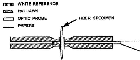
Figure 12. Sketch of the optic fiber probe for thin cotton specimen transreflectance measurements.
