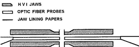
Figure 5. Sketch of optic fiber probes installed in the HVI strength tester.
