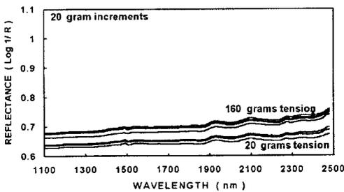
Figure 9. Reflectance spectra of a thin cotton fiber specimen at different bundle tensions.
