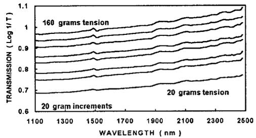
Figure 8. Cotton fiber transmission spectra at different levels of bundle tension.
