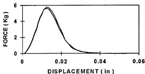
Figure 2. Typical HVI force signals during cotton strength measurements.
