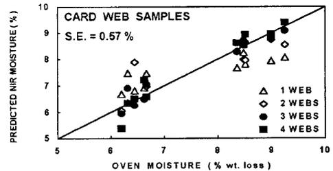
Figure 18. Moisture comparison with four cottons and four fiber web thicknesses.
