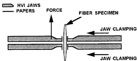
Figure 1. Sketch of the cotton fiber strength measurement.
