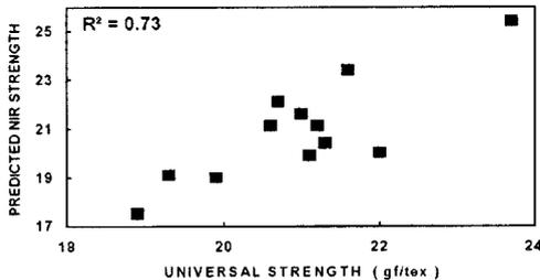
Figure 17. Strength comparison for 12 varieties of cotton using a three wavelength model.
