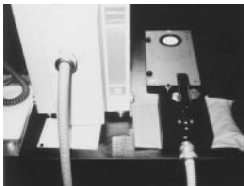
Figure 7. Presentation of fabric sample to NIRS 6500 with fiber optic cable.
