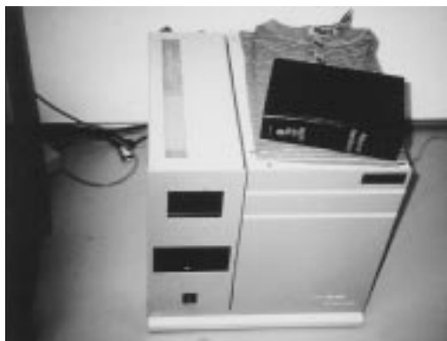
Figure 5. Presentation of garment sample to InfraAlyzer.
