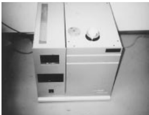
Figure 6. Presentation of fiber, sliver and roving sample to InfraAlyzer.
