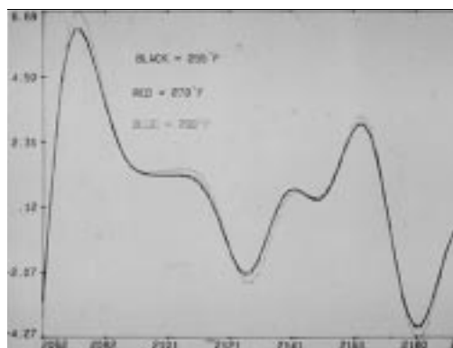
Figure 14. NIR spectra of heat set nylon.
