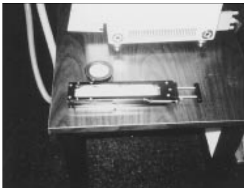
Figure 8. Presentation of fiber, sliver and roving sample to NIRS 6500.
