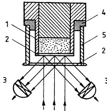
Figure 2. Schematic representation of transreflectance sample holder cell. 1. "Absolute white" powder (reflector). 2. Quartz windows. 3. Lead sulfide detectors. 4. Distance ring for adjustment of sample layer thickness. 5. Sample holder house.
