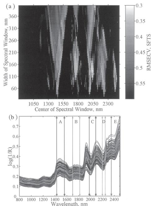
**Figure 3.** Determination of five spectral windows with good performance for prediction of SFTS: (a) three-factor spectral window preprocessing image with the best individual model noted with the symbol  $\otimes$ ; and (b) unprocessed  $-\log[R]$  NIR spectra with indication of the five locally optimal spectral windows A–E. Both plots have the same range of abscissa values.
