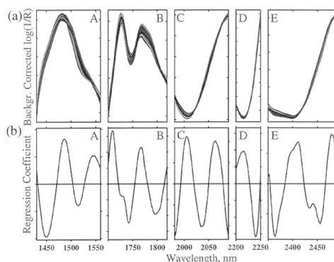
**Figure 4.** Spectral basis of PLSR calibration models for determining SFTS from NIR reflectance of flax stems: (a) background-corrected locally optimal spectral windows A–E; and (b) corresponding regression vectors. The expansion per wavelength is the same for all of abscissa scales. See Table 1 for statistics.
