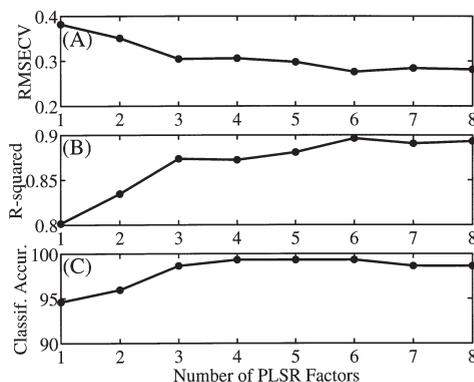
**Figure 2.** Best values among all individual tested NIR spectral windows for PLSR performance statistics v. number of factors, as generated by a cross-validation procedure that preserves the independence of each specimen: (a) *RMS* error in predicting the known SFTS; (b) correlation between predicted and known SFTS; and (c) percent of samples correctly identified as either under- or over-retted. For each statistic the sample retting times ranged from 0 to 14 hours.
