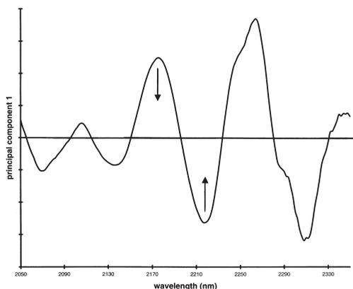
Figure 4.  $\beta$ -lactoglobulin aggregation ( $15 \text{ mg mL}^{-1}$ ). Spectral pattern associated to principal component 1.
