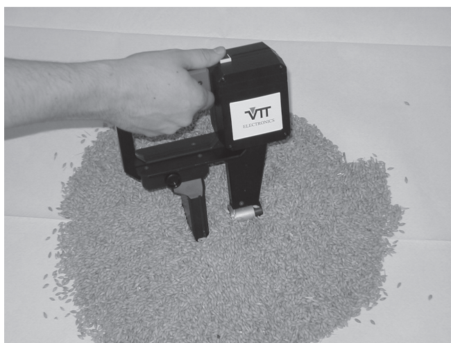
Figure 1. Photograph of GrainGun, the developed hand-held grain analyser.
