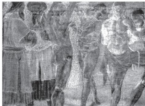
**Figure 7.** Ratio of the 1450 nm image to the 1300 nm image. The areas that reveal gypsum below the painted layer appear as darker zones.
