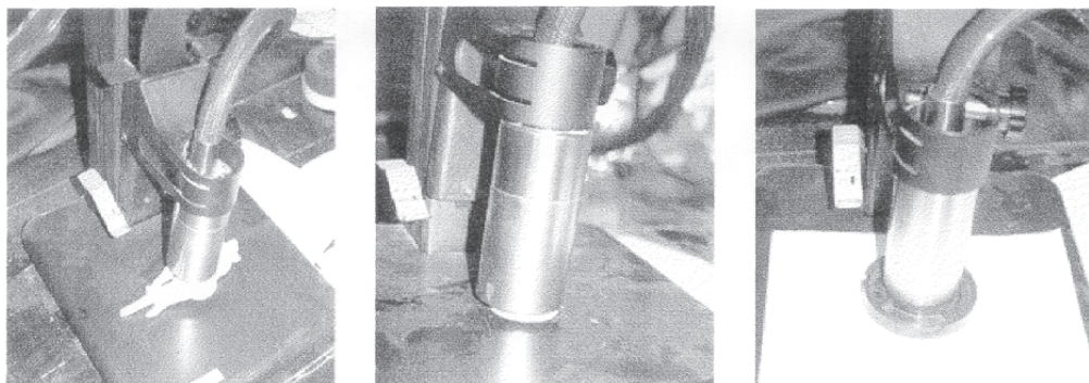
Figure 3. NIR measuring of ginseng radix using a fibre optic.
