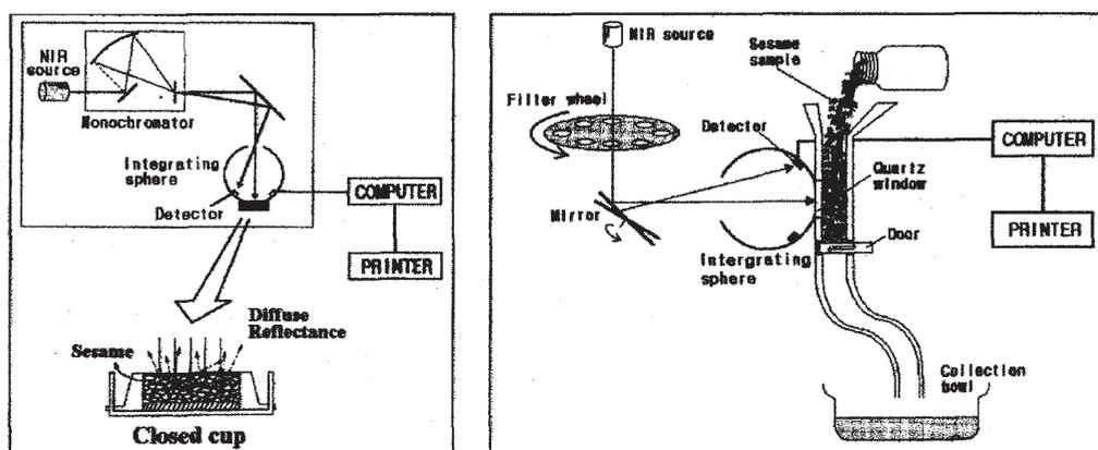
Figure 1. Scheme of NIR spectrum measurement of sesame seed using scanning type (a) and filter type (b) NIR measurements
