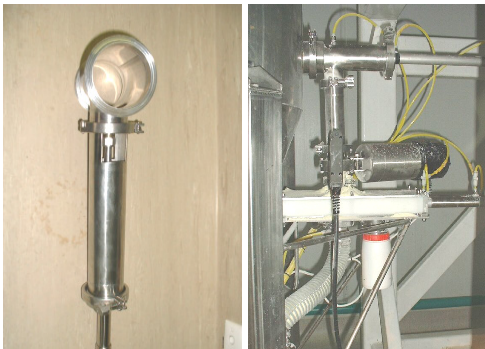
Figure 1. left: butter spool with probe in situ; right: automatic powder sampler for milk powder.
