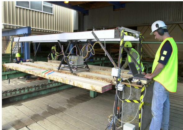
Figure 3. Photo showing the gantry and Matrix-E NIR traversing the cant.
