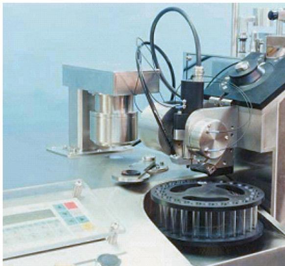
**Figure 3.** On-line NIR analysis of tablets. Tablets are positioned automatically into a customised tablet nest, which is then transferred underneath the NIR reading head. After completion of the NIR analysis tablets are collected in a 25 vial storage carousel.
