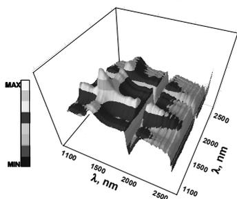
**Figure 1. 3D representation of the synchronous 2D NIR correlation spectrum of the standard process (A).**
