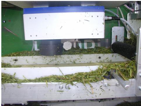
**Figure 2. Conveyor belt mounted at the rear of a forage harvester under the diode array spectrometer.**
