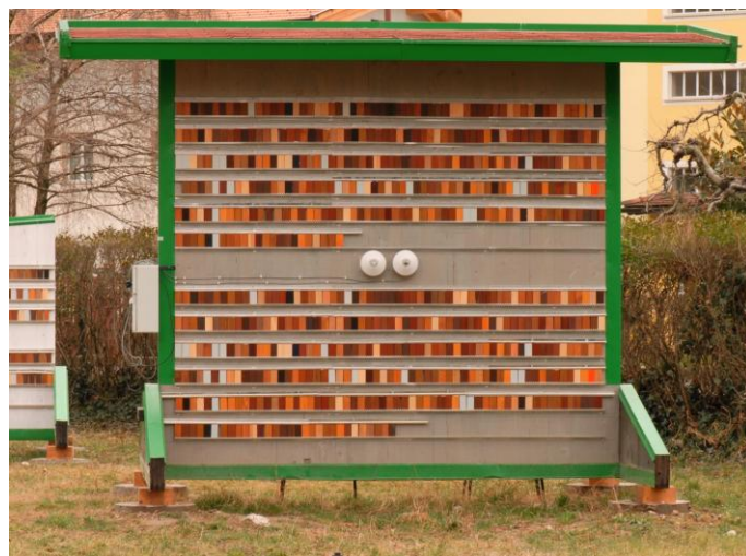
Figure 1. Field stand for holding experimental samples during natural weathering test.
