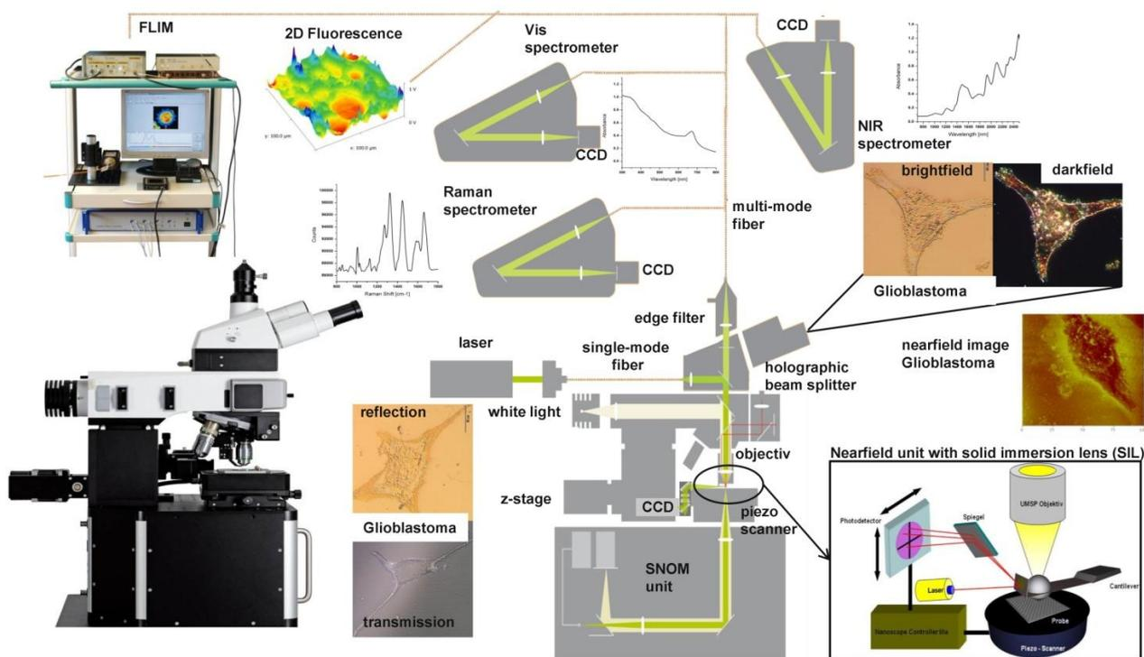
**Figure 5.** New concept for multimodal hyperspectral near-field imaging and spectroscopy: fast scanning whiskbroom imaging system on the basis of a WITec microscope with solid immersion lens for near-field measurements.
