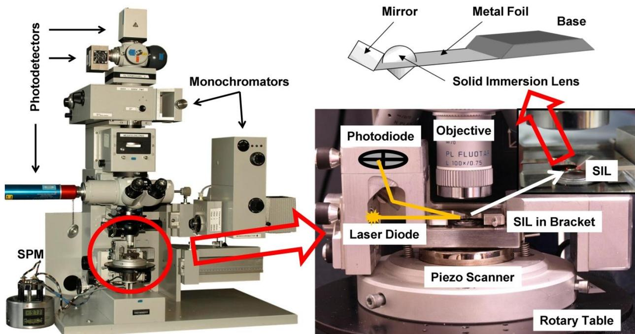
**Figure 2.** System Integration. Left: Zeiss Universal micro-spectrophotometer (UMSP 80) with SIL unit mounted underneath the objective. Right bottom: SIL cantilever on top of a piezo scanner with laser beam path for deflection measurement. Right top: SIL glued in metal foil cantilever with side mirror.
