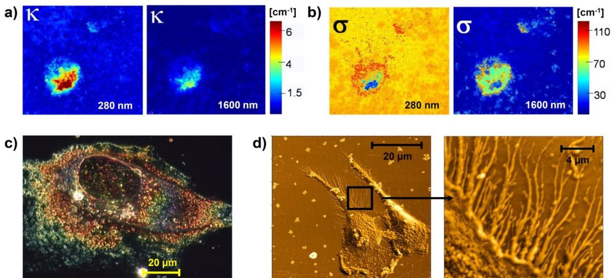
**Figure 4.** Trade-off between scatter and absorption. a) and b) calculations of absorption coefficient  $\kappa$  and scattering coefficient  $\sigma$ , respectively, at 280 and 1600 nm of an active pharmaceutical ingredient surrounded by the excipient of a tablet. c) Microscopic dark-field RGB image of a glioblastoma multiforme cell, fixed with paraformaldehyde. d) Vis-SIL near-field images of a monocyte with dendritic branches.
