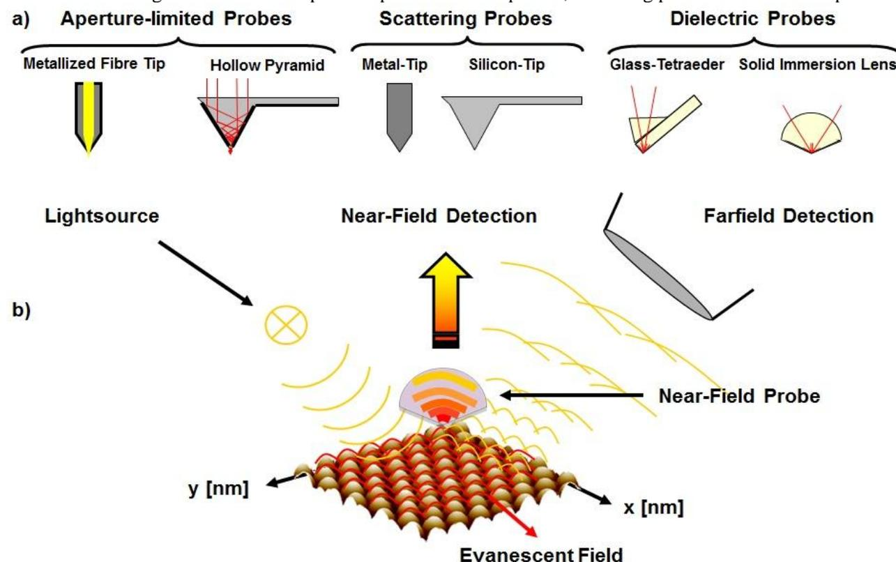
**Figure 1.** a) Examples of near-field probes: aperture-limited probes, scattering probes and dielectric probes. b) Near-field concept using a SIL as a nanoprobe for the conversion of evanescent waves to propagating waves.
