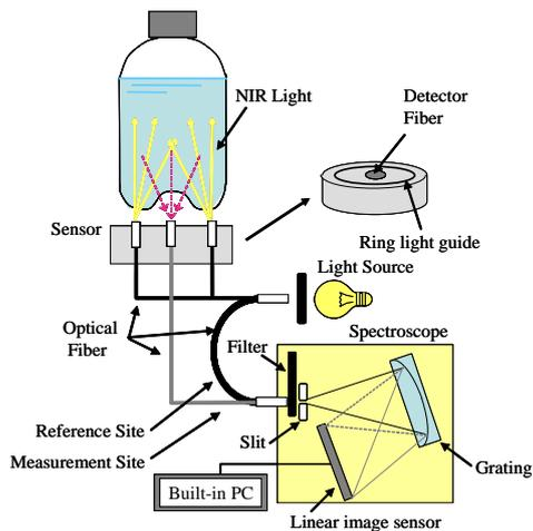
Figure 1. Schematic figure of a NIR bottle scanner.
