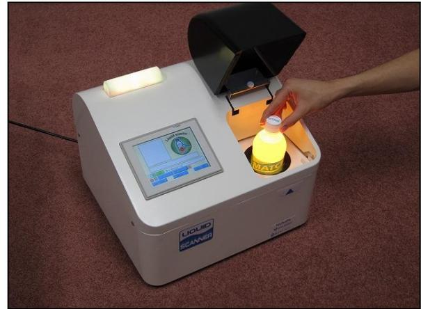
Figure 2. Photograph of a NIR bottle scanner.
