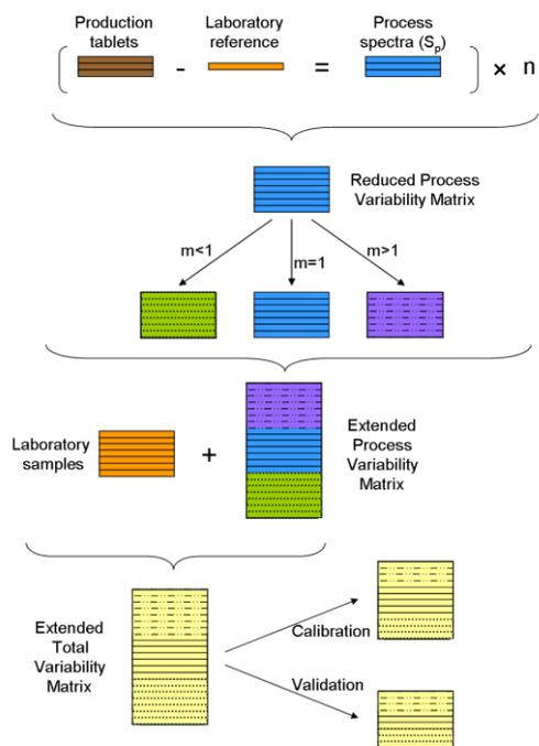
**Figure 1.** Calculation of the process spectrum.
