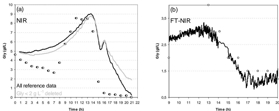
**Figure 4.** *E. coli* fermentation process accumulation profile for Gly (g·L<sup>-1</sup>). NIR predicted values are lines smoothed by ten-point moving averages and reference chemical assays are circles.
