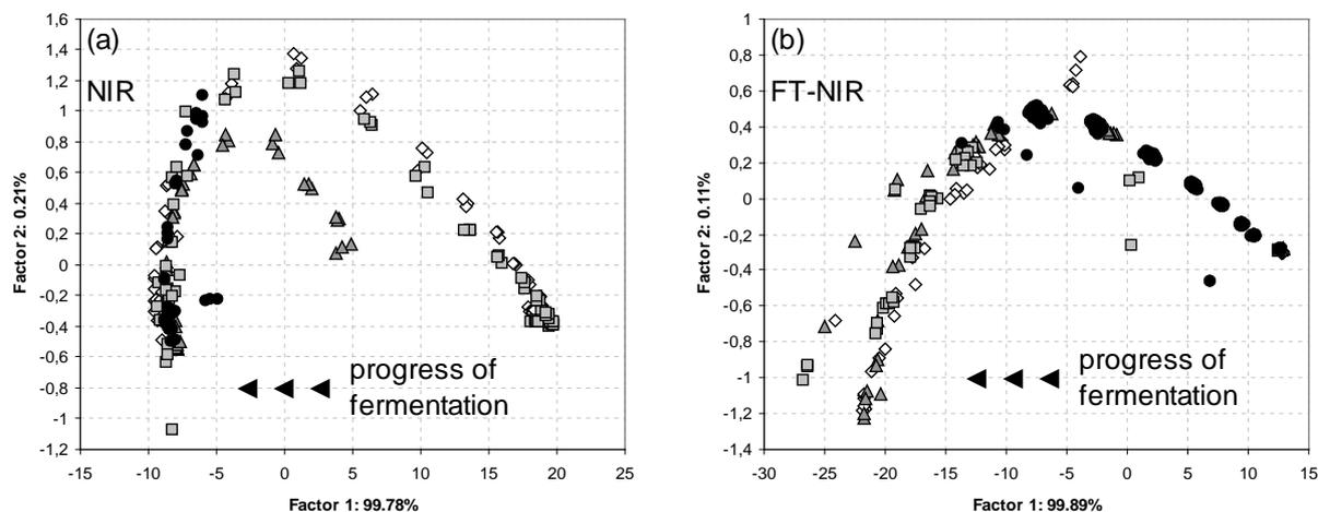
**Figure 2.** PCA score plots of 3<sup>rd</sup> overtone (700–1100 nm) spectra from fermentation batches F\_1 (◇), F\_2 (▲), F\_3 (□), F\_4 (●) (Figure 2a) and F\_5 (◇), F\_6 (▲), F\_7 (□) and F\_8 (●) (Figure 2b). Each point represents a spectrum from a time point of the run.
