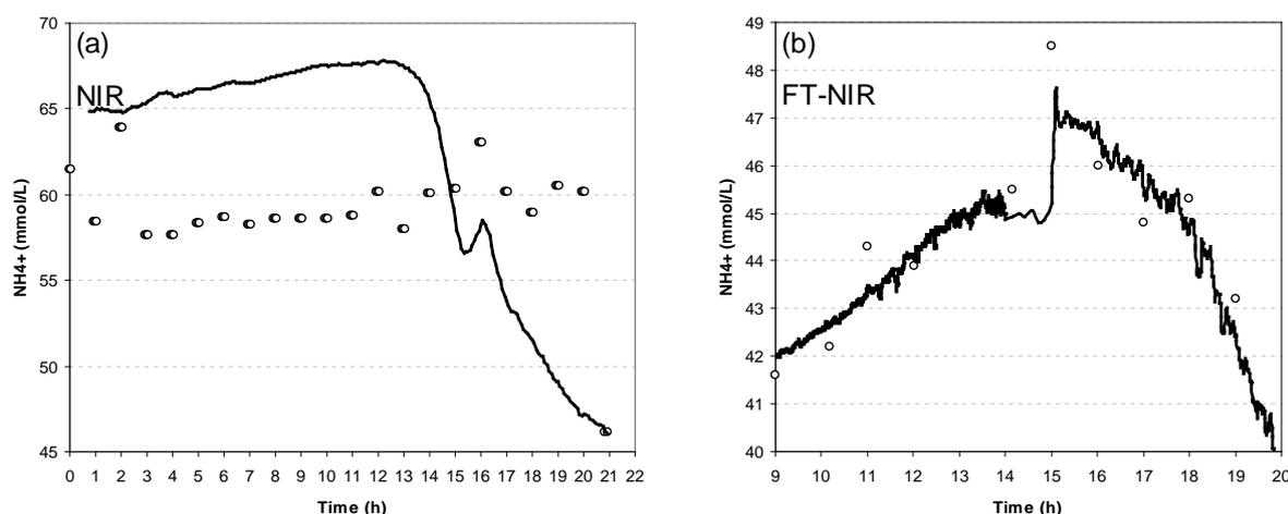
**Figure 5.** *E. coli* fermentation process accumulation profile for NH<sub>4</sub><sup>+</sup> (mmol L<sup>-1</sup>). NIR predicted values are lines smoothed by ten-point moving averages and reference chemical assays are circles.
