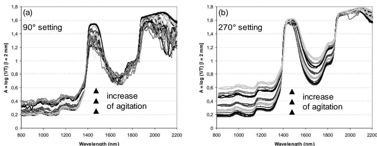
**Figure 1.** NIR spectra of glycerol-water mixture using 400 600, 800, 1000, 1200, 1400, 1600 and 2000 rpm agitation in the case of  $90^\circ$  (Figure 1a) and  $270^\circ$  (Figure 1b) settings.
