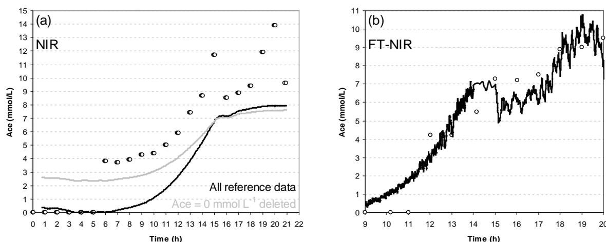
**Figure 3.** *E. coli* fermentation process accumulation profile for Ace (mmol.l<sup>-1</sup>). NIR predicted values are lines smoothed by ten-point moving averages and reference chemical assays are circles.
