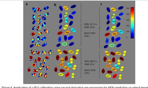
Figure 4. Application of a PLS calibration using second derivative pre-processing for HFN prediction on wheat kernels by HSI, by using two methods: a) pixel-by-pixel application of the calibration and b) average calculation of the predicted HFN; c) application of the calibration on the mean NIR spectrum for each kernel. HFN: predicted value for the batch; SEM: standard error of the mean; Batch HFN: reference measurement value. Numbers on wheat kernels indicate the predicted HFN (s).
