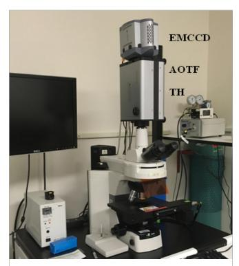
Figure 1. Hyperspectral microscope imaging system.
