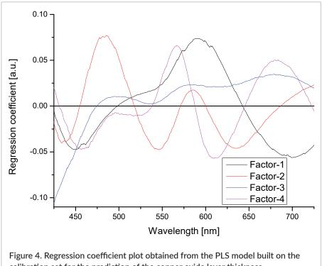
calibration set for the prediction of the copper oxide layer thickness.
