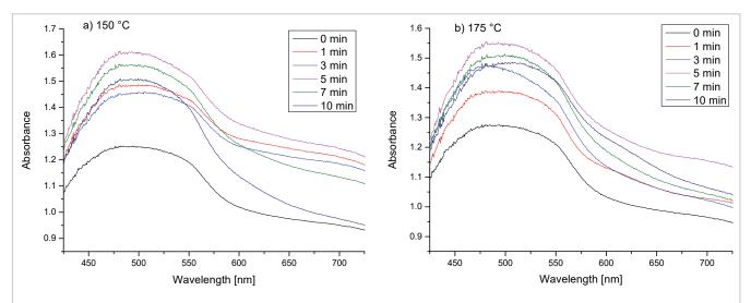
Figure 1. Reflectance spectra obtained by averaging 13,000 spectra in the wavelength range from 425 nm to 725 nm of copper substrates oxidised at a) 150 °C and b) 175 °C. The oxidation time of each sample is given in minutes.
