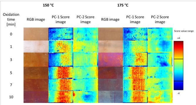
Figure 2. Score and RGB images of copper substrates obtained from the calibration set, oxidised at different times and temperatures. The coloured pixels represent the oxide content, from low (blue) to high (red). The black squares show the area for calculation of the average spectra for each sample (PC1 92.9%, PC2 4.12%).
