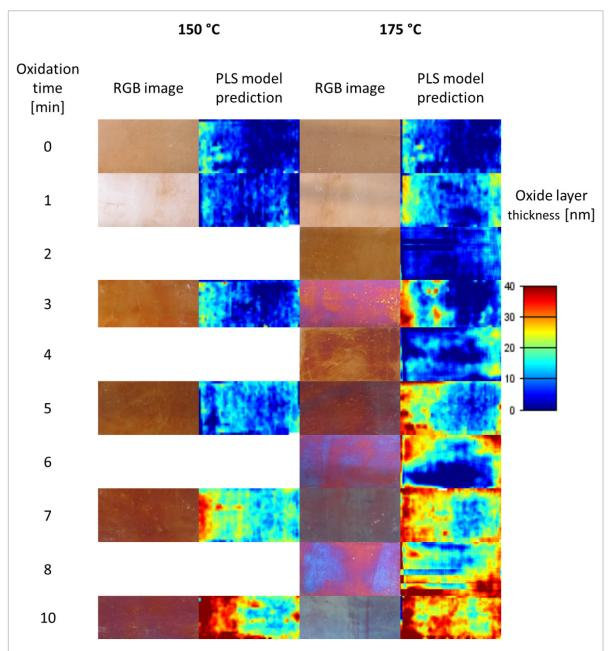
Figure 6. Predicted oxide layer thicknesses and RGB images for the copper substrates from the prediction and calibration set, oxidised at different times.
