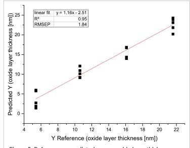
Figure 5. Reference vs predicted copper oxide layer thicknesses plot based on the external validation set.
