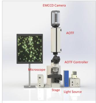
Figure 2. The hyperspectral microscope imaging system. Note: EMCCD = electron multiplying charge coupled device, AOTF = acousto-optic tuneable filter.
