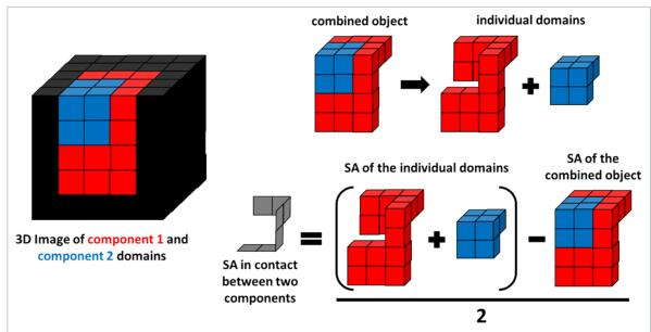
Figure 3. A schematic of the 3D domain adjacency process. The SA in contact between domains of two components is calculated by determining the SA of the individual single component domains and the combined two-component object.
