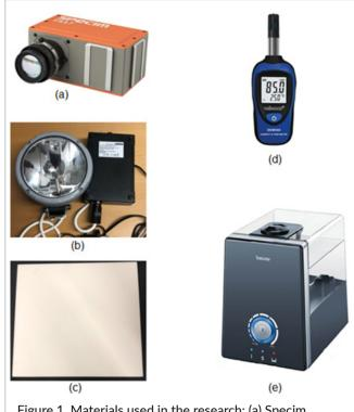
Figure 1. Materials used in the research: (a) Specim FX17e hyperspectral camera, (b) Rallye 3003 compact halogen lamp, (c) PTFE tile, (d) DEM500 humidity sensor, (e) Beurer Gmbh's LB 88 humidifier.
