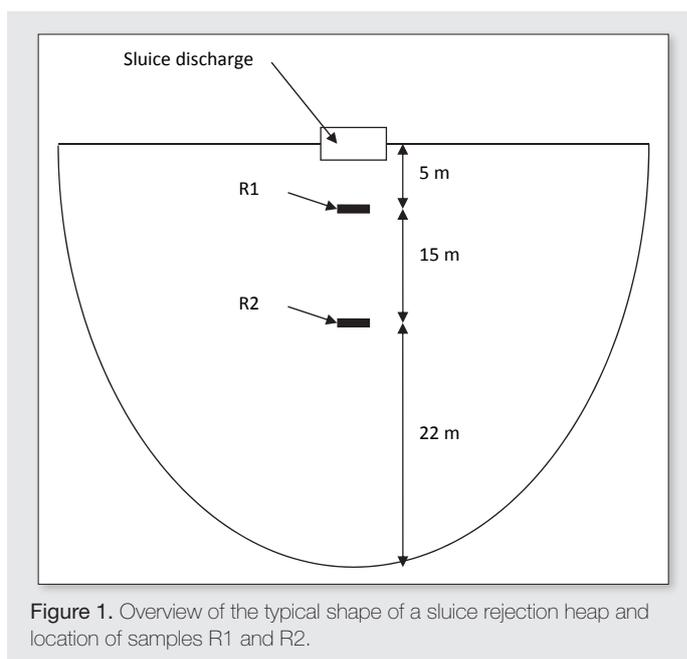
Figure 1. Overview of the typical shape of a sluice rejection heap and location of samples R1 and R2.
