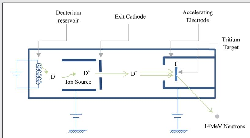
Figure 2. Neutron Tube Principle
